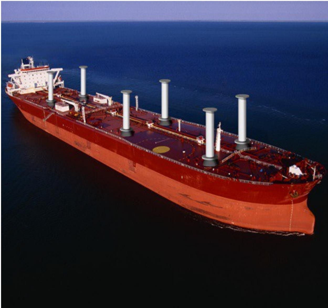
Adapting Flettner rotors so thrusting bases can generate power for a green ammonia plant on board - as set out in a not-yet-published patent application of mine - removes the need for many wind farms altogether. Just send shuttle tankers to where the winds are and return when the ammonia tanks are full.
