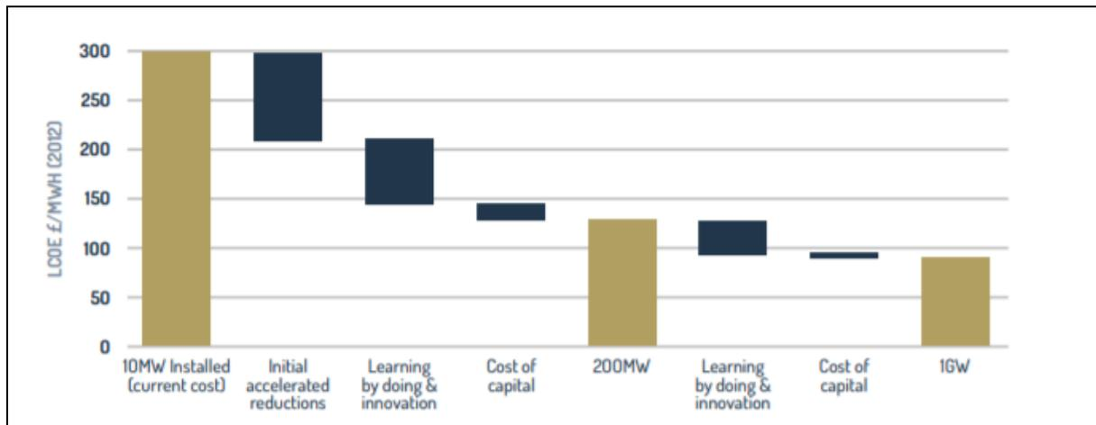
Figure 4 - Tidal Stream LCoE reduction
