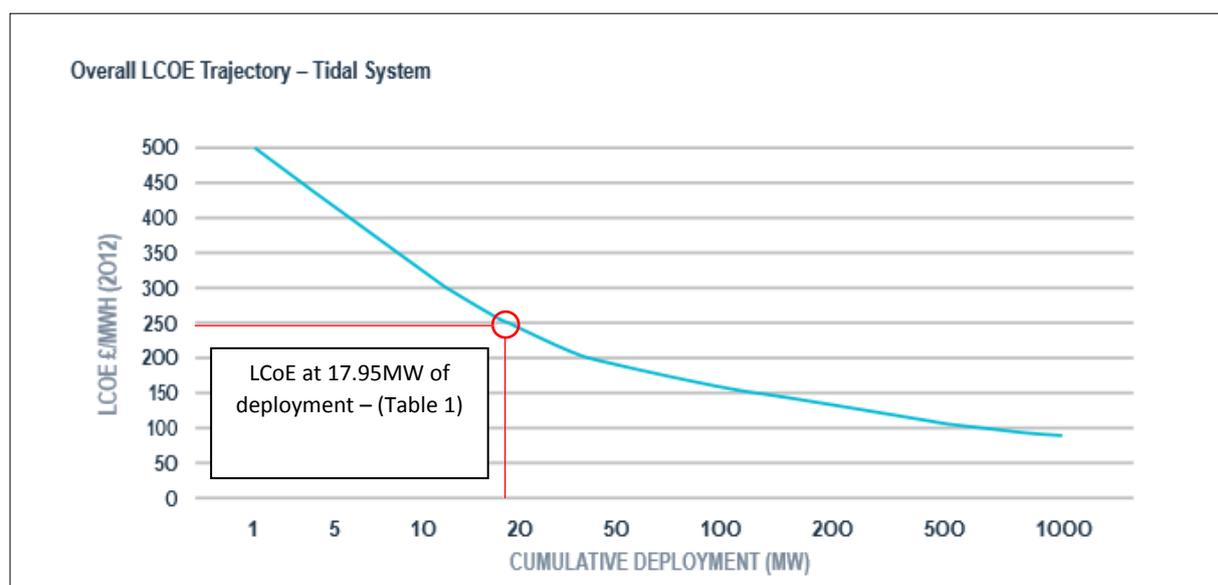
Figure 3 - Tidal stream estimated trajectory to 1GW<sup>5</sup>
