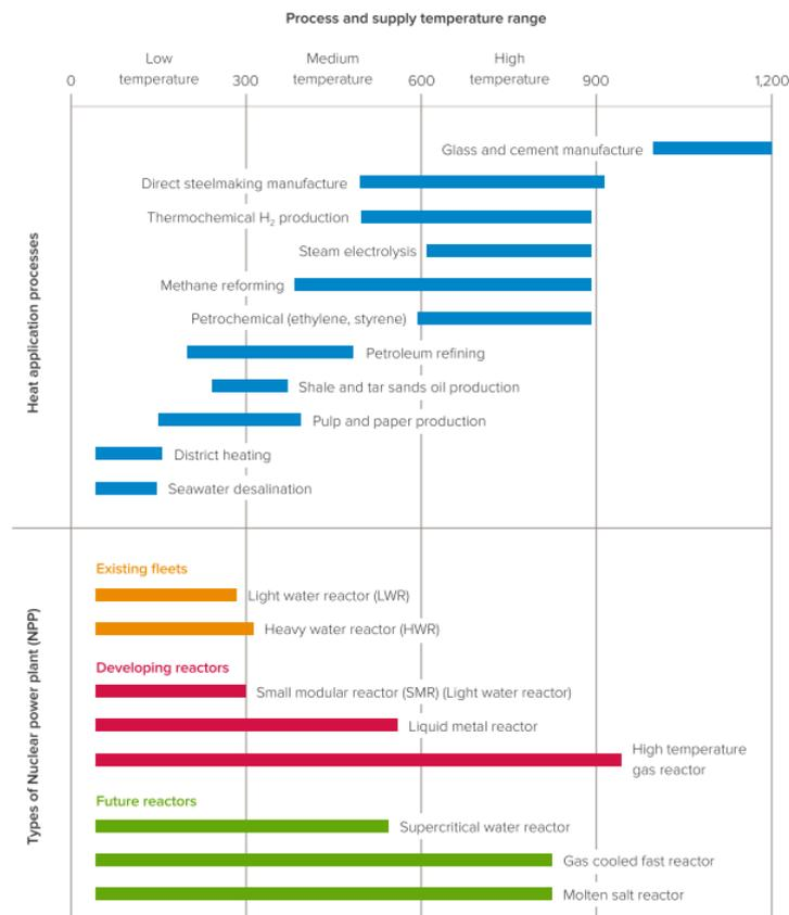
Figure 2. Temperature ranges of heat application processes and types of nuclear power plant [7, Fig. 6].
