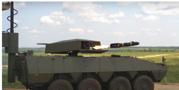
Figure 3: AGM-114 Hellfire (Helicopter Launched Fire-&-Forget Missile System) integration and firing with Lockheed Martin UK turret on a Patria AMV 8x8 base vehicle platform for a potential export customer (2014)
