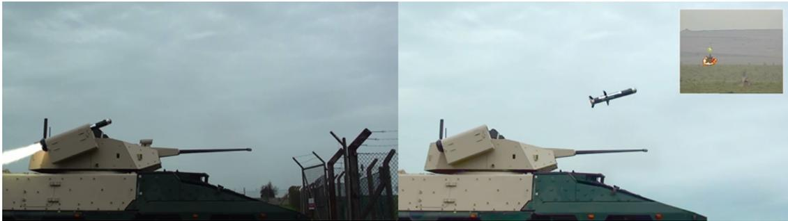
Figure 1: FGM-148 Javelin ATGM integration and firing with Lockheed Martin UK turret on a KMW Boxer 8x8 base vehicle platform for a potential export customer (2014-15)
