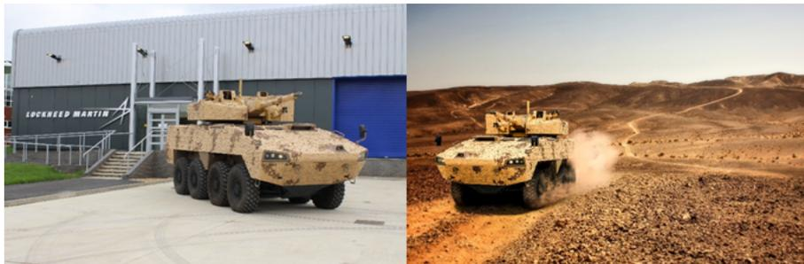
Figure 2: FGM-148 Javelin ATGM integration with Lockheed Martin UK turret on a Patria AMV 8x8 base vehicle platform for a potential export customer (2015-17)
