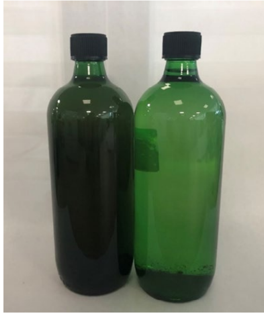
Figure 5: Sample bottles of run-off (L) before and (R) after treatment through a rain garden in the Grangetown SuDS project.
