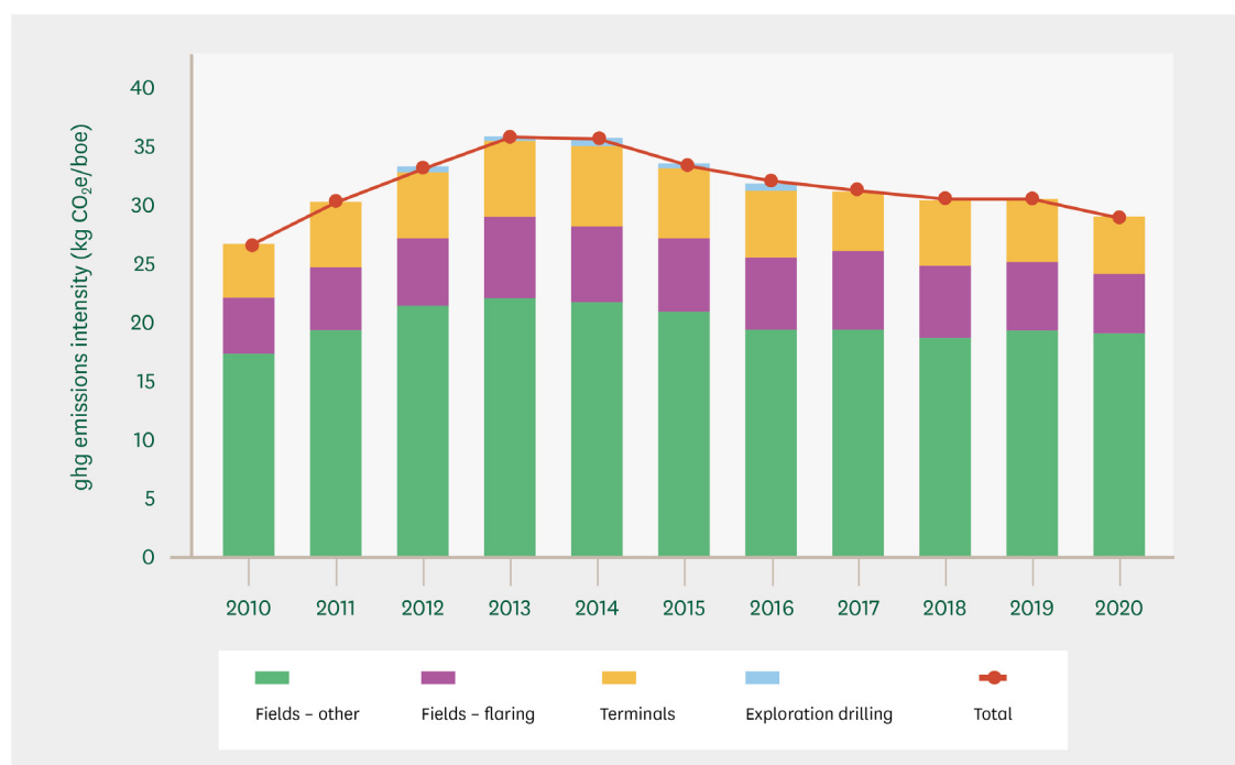
Figure 3: UK Continental Shelf GHG emissions intensity for oil and gas by source and total, 2010–2020
