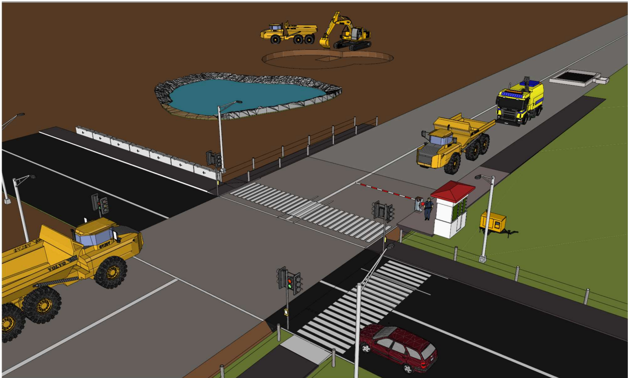
Figure 2 - Illustration of typical plant crossing
