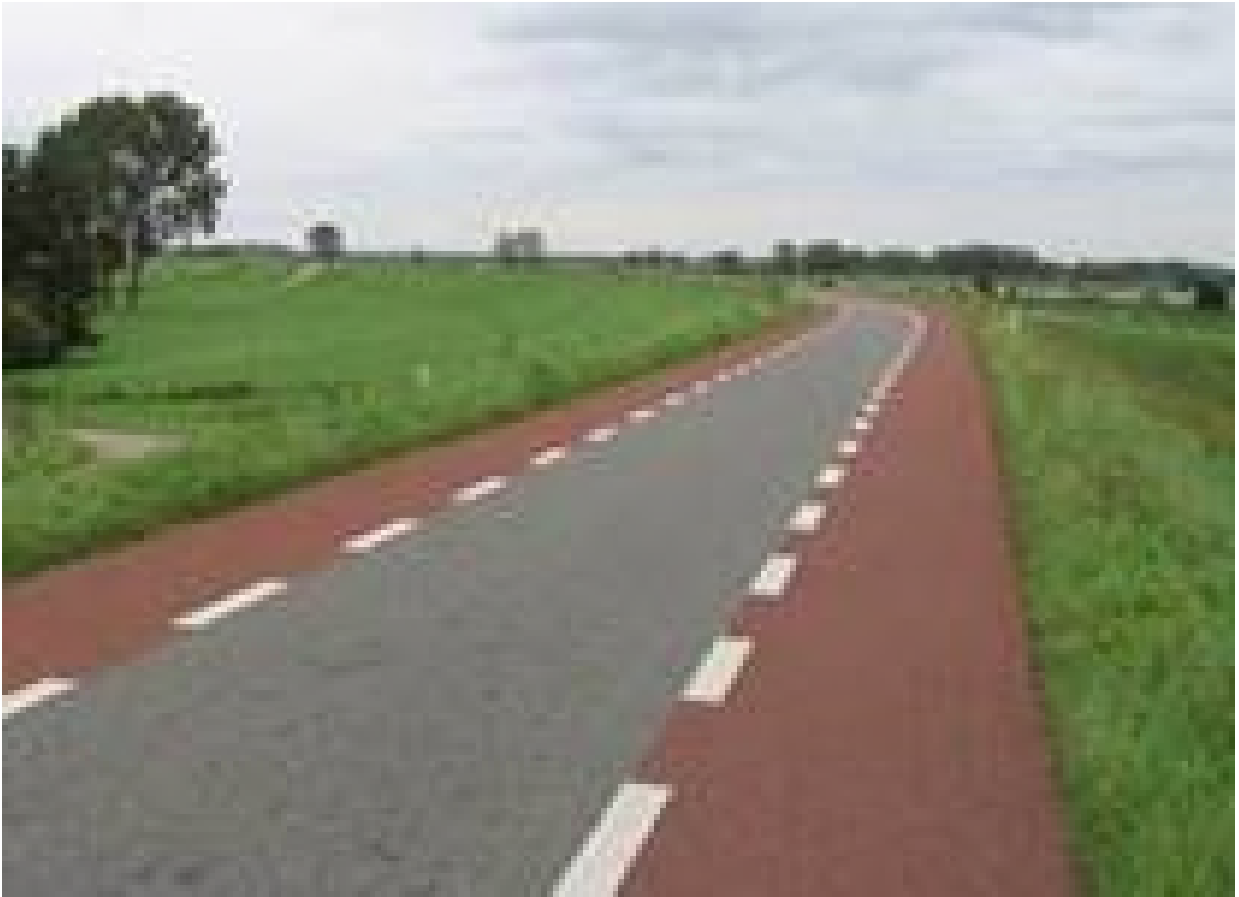
Dutch example of 60km/h rural lane with cycle lanes and no centre lines
