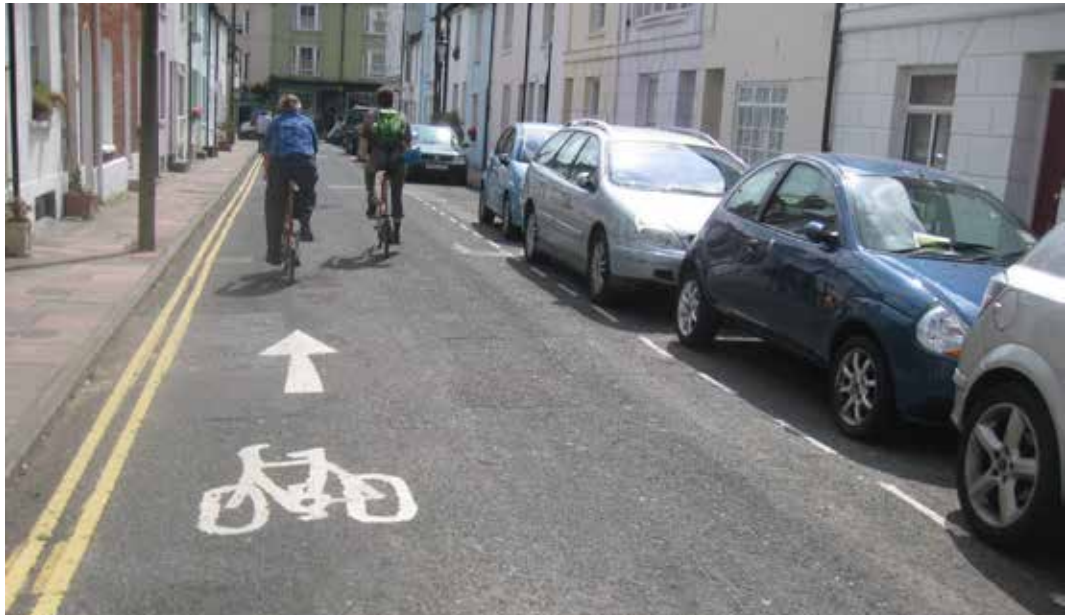
Photo 6.5 - Contraflow cycling in a narrow street with no marked lane – Brighton
